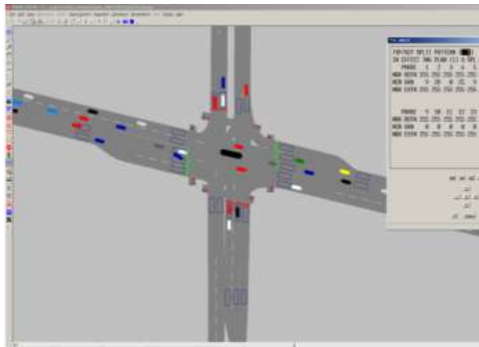
TSP Corridor VISSIM Model with ASC/3 Signal Controller
